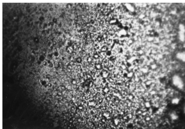
Figure 5 Scanning electron micrograph of the biodegraded film of the PP/AM/DODAM (70/25/5) blend.
